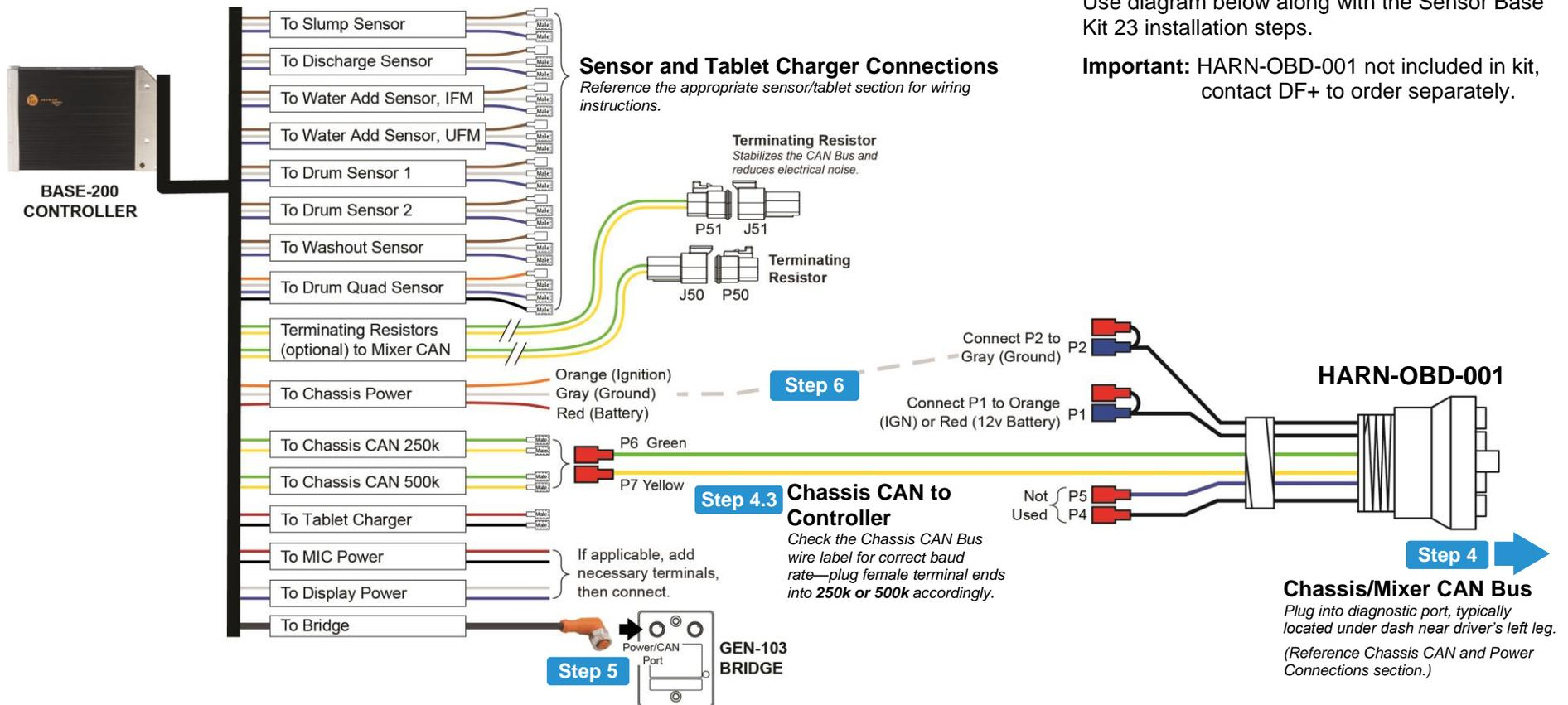
Use diagram below along with the Sensor Base Kit 23 installation steps.
