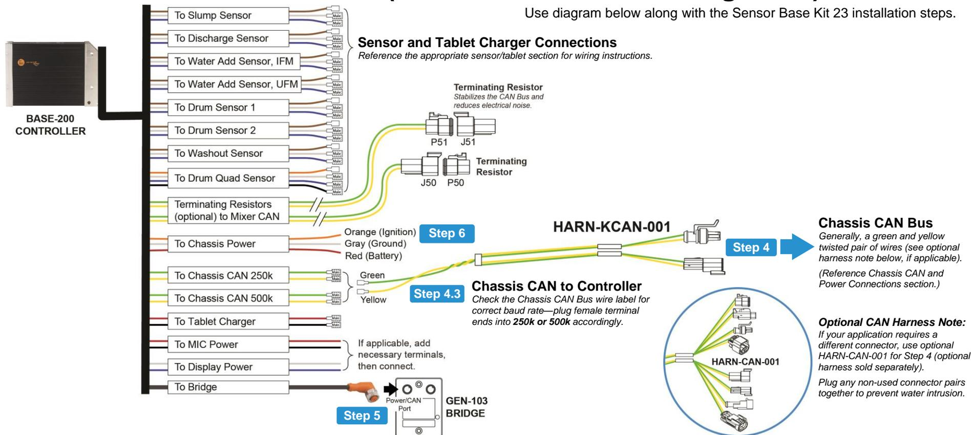
**Step 4. Connect Controller to Chassis CAN Bus (use HARN-KCAN-001)**
