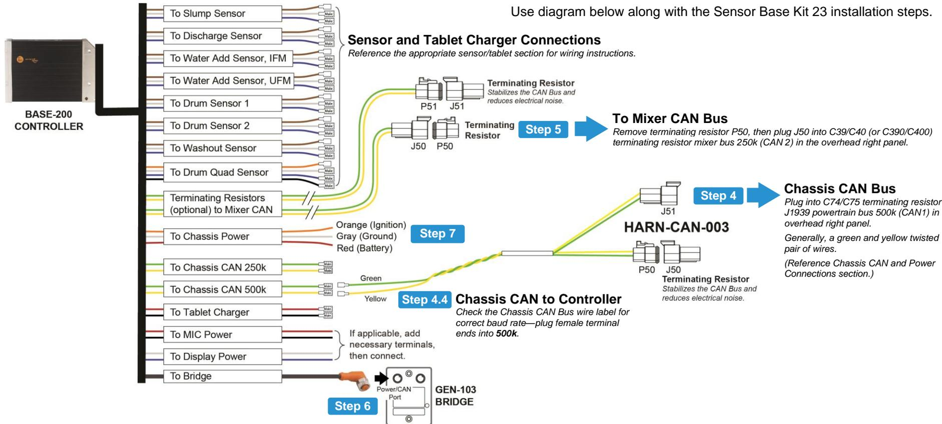
**Step 4. Connect Controller to Chassis CAN Bus (use HARN-CAN-003)**
