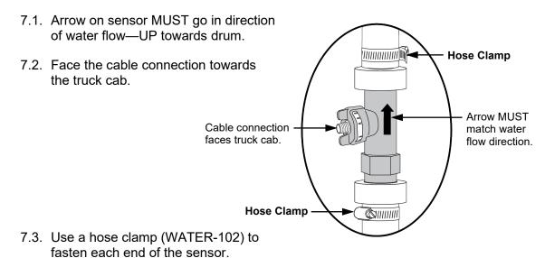
Fasten hose securely to avoid leaks.
