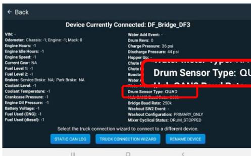
4.3 **Parameter setting**—scroll down on diagnostic screen to observe drum sensor type, it should read QUAD (*If incorrect, call DF+ Support.*)
