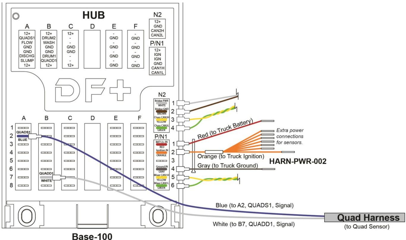
**Step 3.** Double check that all wiring connections are securely fastened.
