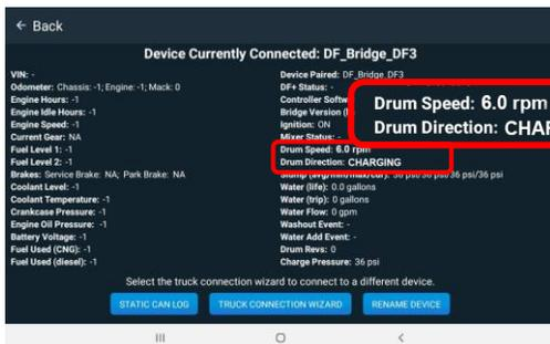
4.2 On diagnostic screen—observe drum speed and direction during the following tests:
