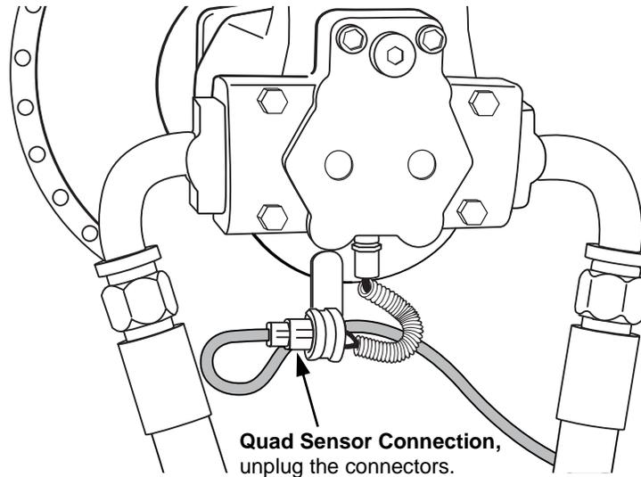
**Step 4.** Connect the Quad Harness provided in the kit—you will have either a HARN-QUAD-001 (for McNeilus), or HARN-QUAD-002 (for Con-Tech).
