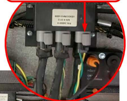
Figure A: 6-way Chassis CAN Connector —If 6-way bus not plugged in here, see Figure B for 3-way Gray Splitter.
