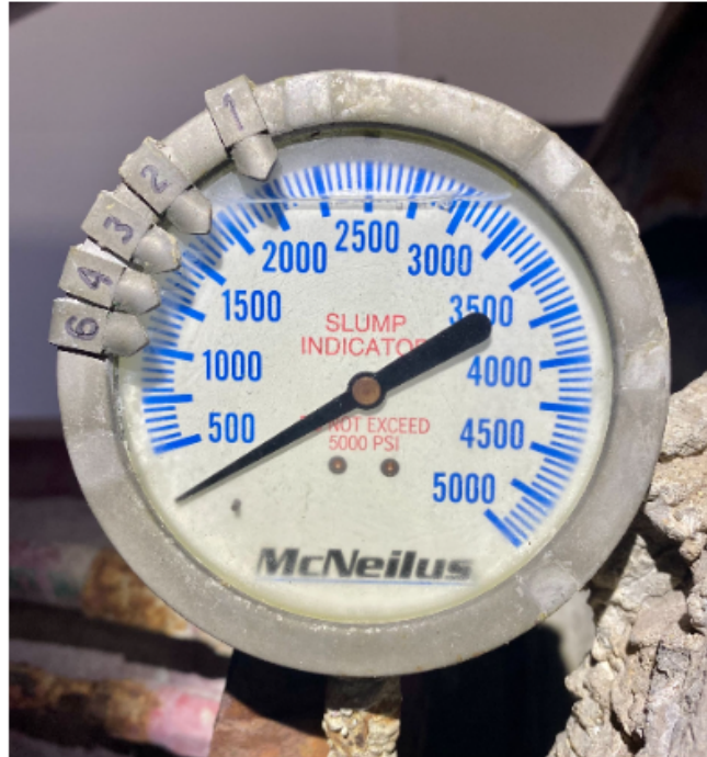
Figure 1: Hydraulic Charge Pressure Gauge with Slump Inch Markers
